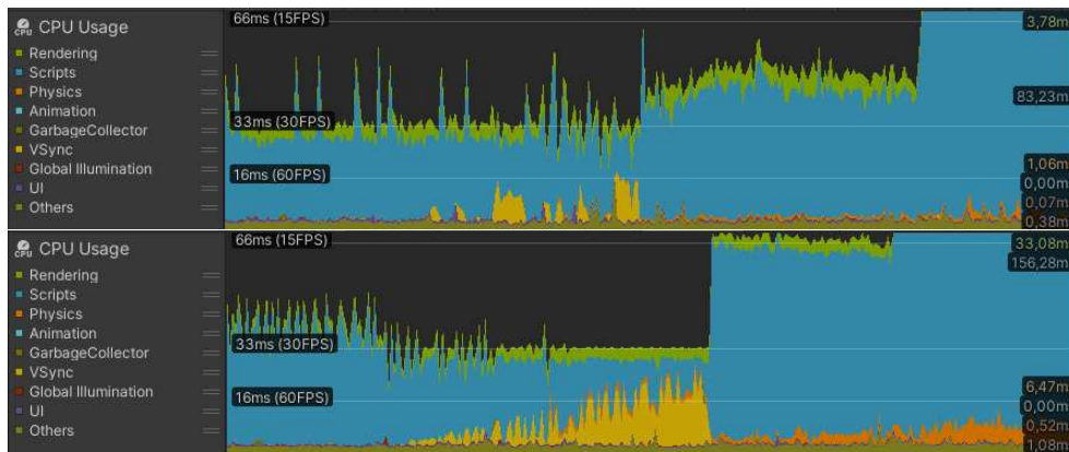
Figure 3.11: Performance graphs of the OnePlus Nord (top) and Google Pixel 3a XL (bottom) devices from the Unity Profiler [28]. The graphs show the application going through a simple scenario: detect surface, place 3D model, and enlarge the 3D model so that it takes up most of the screen. The individual steps are clearly noticeable in the graphs as they cause a significant drop in the frames per second (FPS) measure (the measure increases from top to bottom in the graph). The OnePlus device performs measurably better, but both devices dip into single-digit framerate in the worst-case scenario. Note: the graph is labeled as CPU Usage. This is because Unity reports GPU usage as CPU usage in mobile devices.
