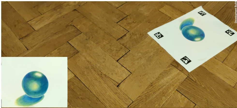
Figure 3.8: A screenshot from the ScannerTest scene, demonstrating the scanner’s functionality. The bottom-left corner shows the result of the perspective transformation.
