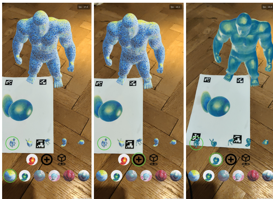
Figure 3.6: The scanning flow is demonstrated in three steps from left to right: (1) place an object, (2) click the plus button, and (3) make sure all four markers are visible.
