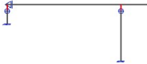
Figure 24: Model for short-term loads during construction – stage 1
