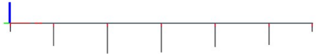
Figure 82: Torsion moment M_x : Differential temperature load
