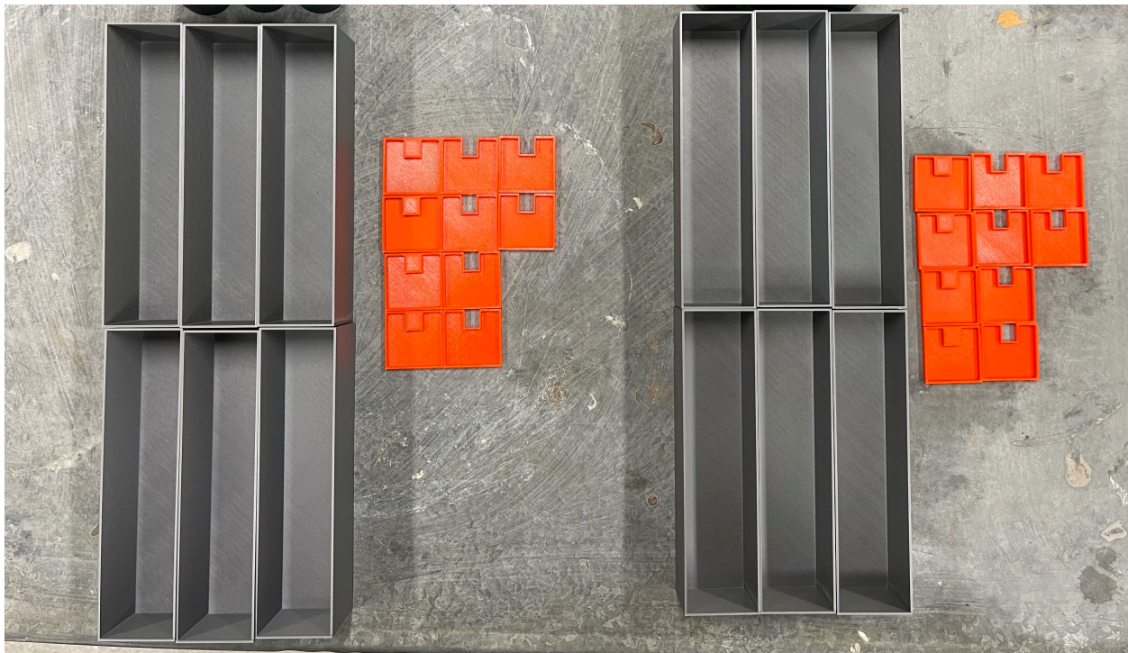
Figure 18. Molds for concrete samples.
