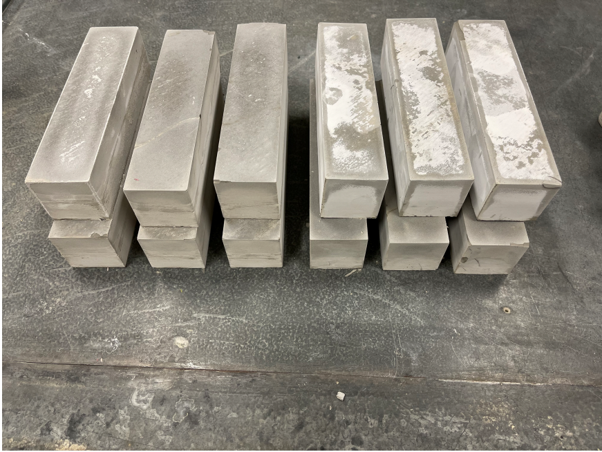
Figure 29. Samples for tensile and compressive strength tests.
