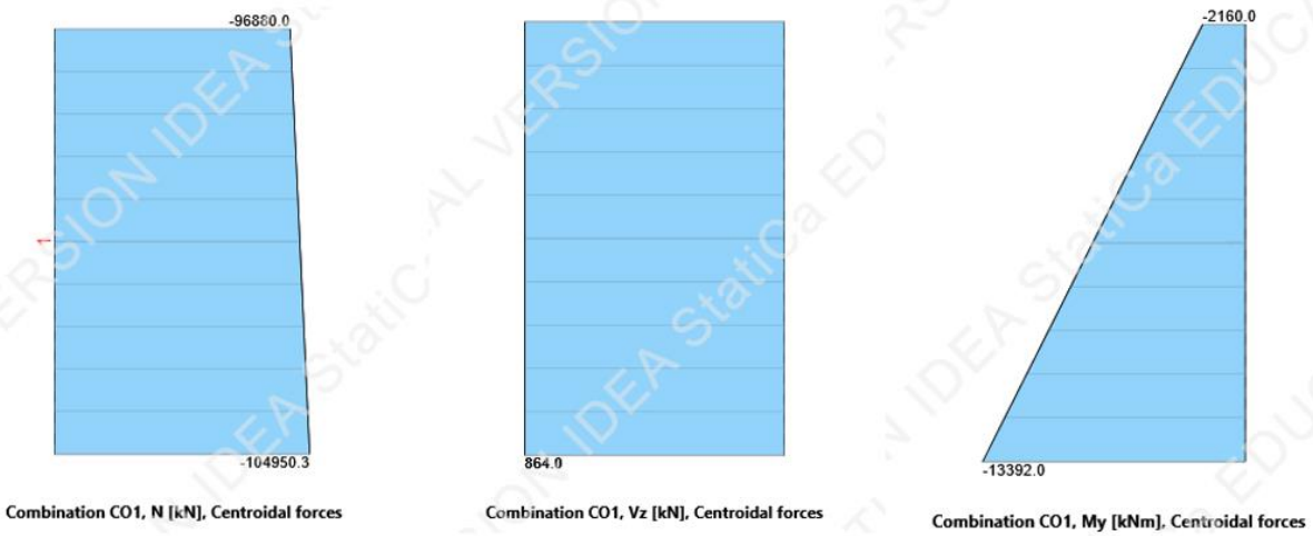
Figure 275 Design action used for pier
