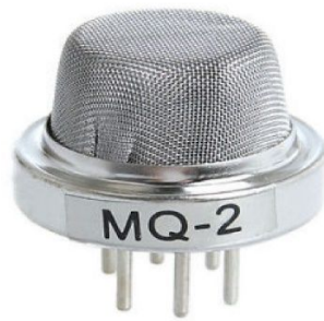
FIGURE 4.3: Smoke Sensor [XXI]
