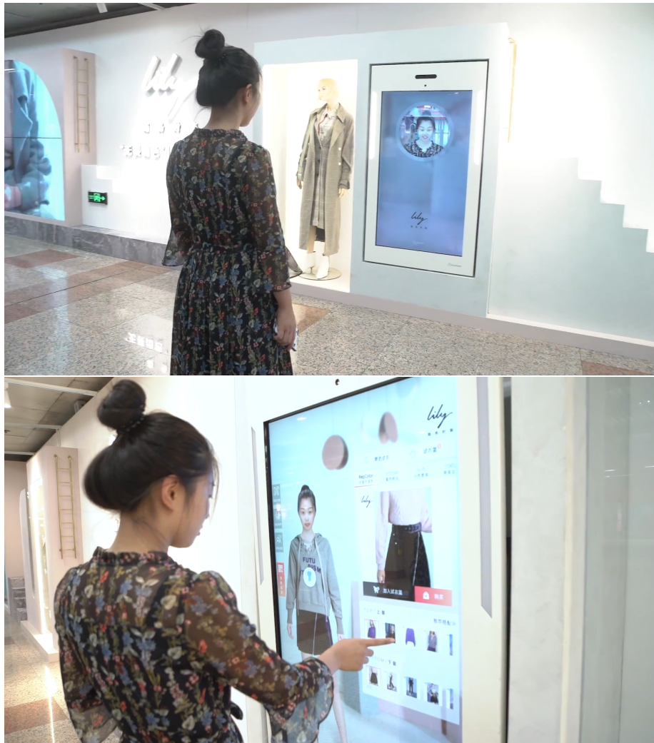
Figure 2.4: Example of virtual clothes fitting in 3D with a customized avatar made with user scanning. Virtual fitting room of brand Lily at in Shanghai metro. Source video: [10].
