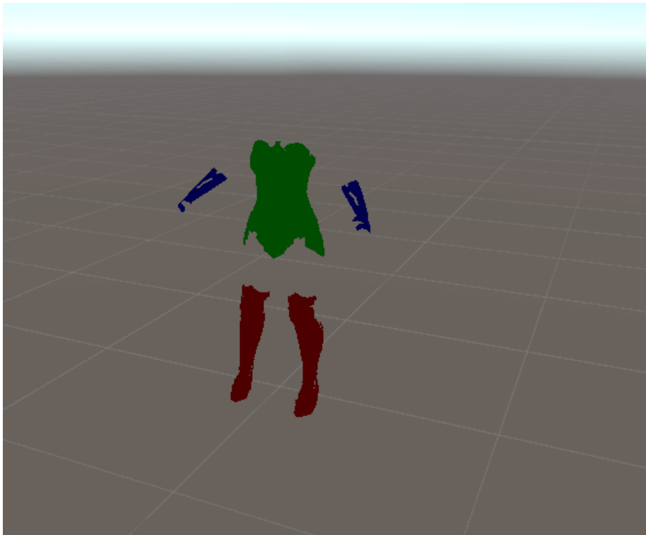
Figure 4.26: Demonstration of the stencil buffer after rendering each piece of clothing. Colors represent the state of the stencil buffer.
