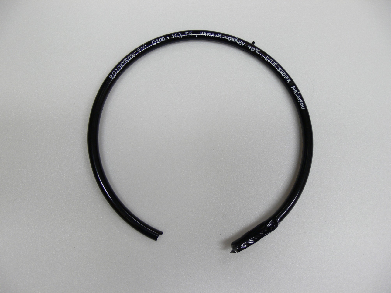
Large core, heated mould casting, 90 Epox + 10 Magnetit:
