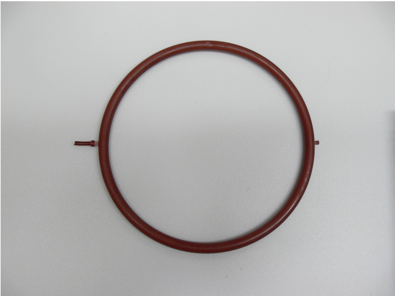
Large core, mould casting, Epox + Nickel-zinc-ferrite:
