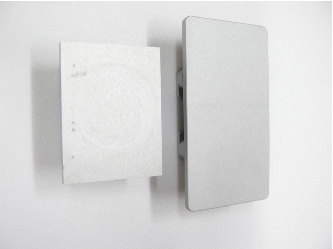
Medium core, mould casting, 80 Epox + 20 Fe:
