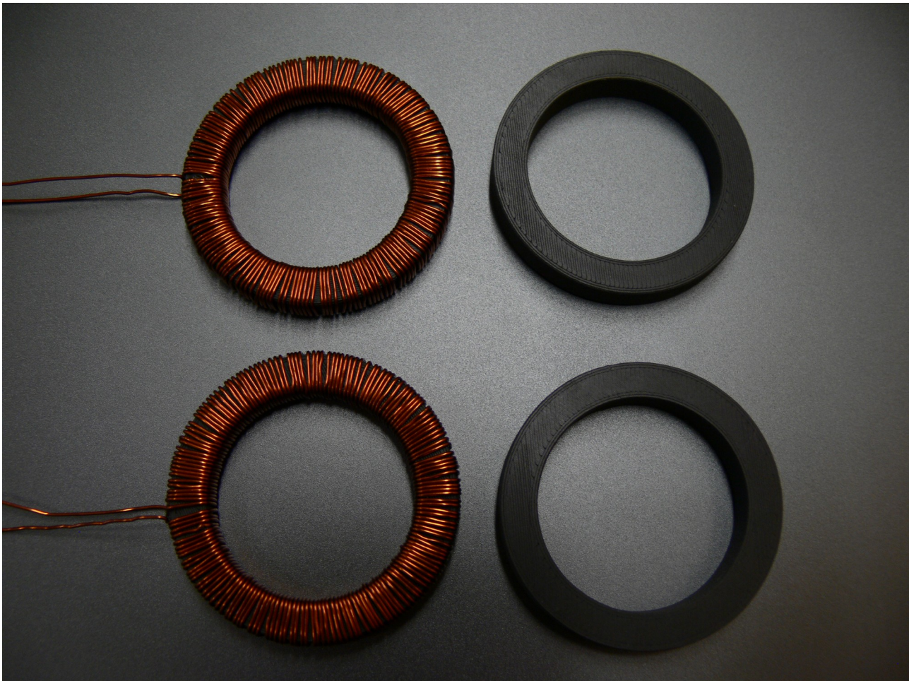
Small cores, 3D printed, Protopasta filament:
