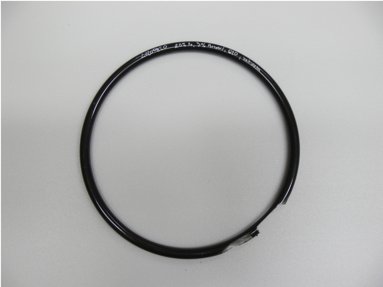
Large core, vacuum mould casting, 80 Epox + 20 Fe:
