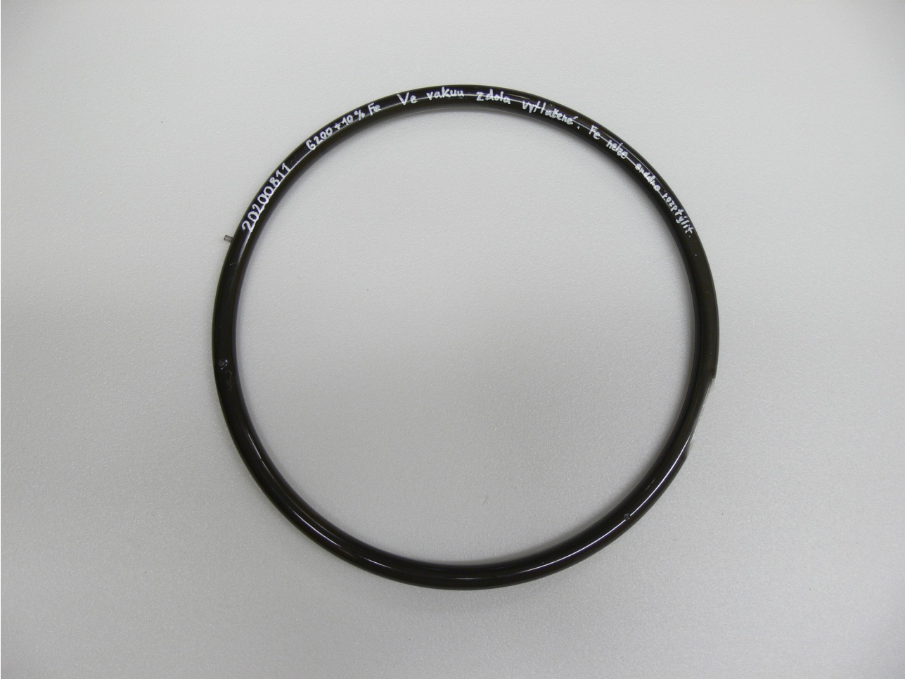
Large core, vacuum mould casting, 90 Epox + 10 Fe:
