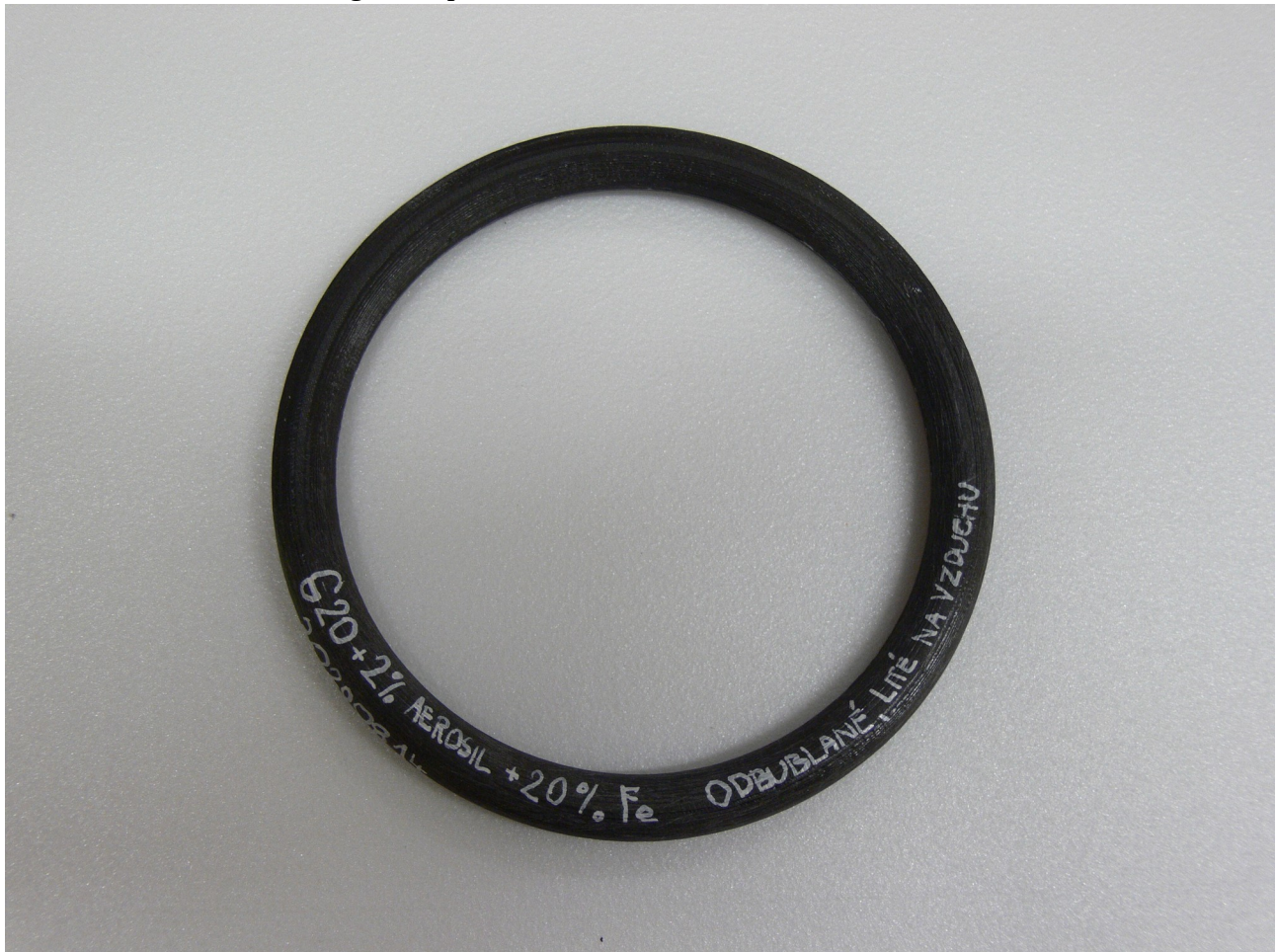
Medium core, mould casting, 80 Epox + 20 Fe:
