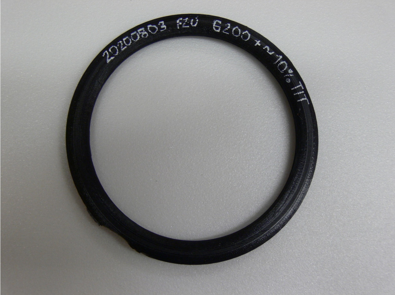
Medium core, mould casting, 90 Epox + 10 Magnetit:
