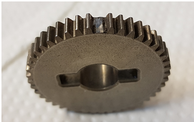
Figure 3.1: Gear broken tooth from our experiment
