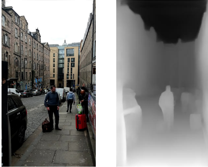
Figure 2.1: Depth estimation of a scene by Megadepth CNN. The original image on the left and the depth map visualized as a grayscale image on the right.
