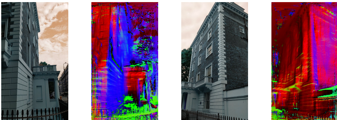
Figure 2.2: Visualization of surface normals as computed via the weighted SVD. The (x, y, z) components of the unit normals correspond in order to the blue, green and red channel respectively.
