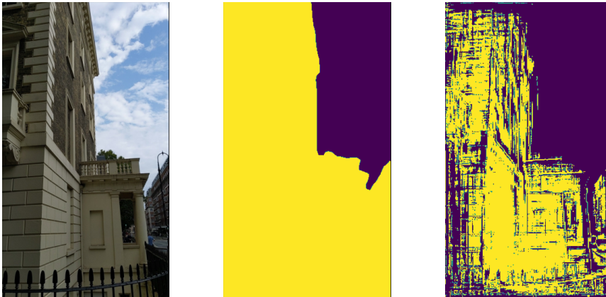
Figure 2.3: Sky filtering and filtering based on the singular values ratio. From left to right: original image, sky mask and mask based on singular values ratio on top of the sky mask ( \alpha_q=0.6 used). Yellow pixels are considered for further processing (normals clustering), ultra violet pixels are ignored.
