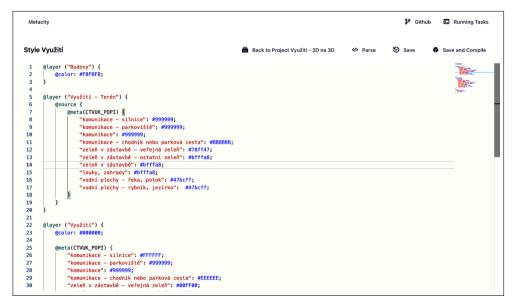
Figure D.13: The style editor utilizes the monako-editor library developed by Microsoft; the editor supports defining custom rules for code completion.
