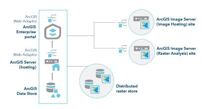
Figure 4.5: ArcGIS Enterprise deployment pattern [68]
