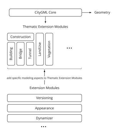
Figure 4.3: Simplified CityGML Module Overview
