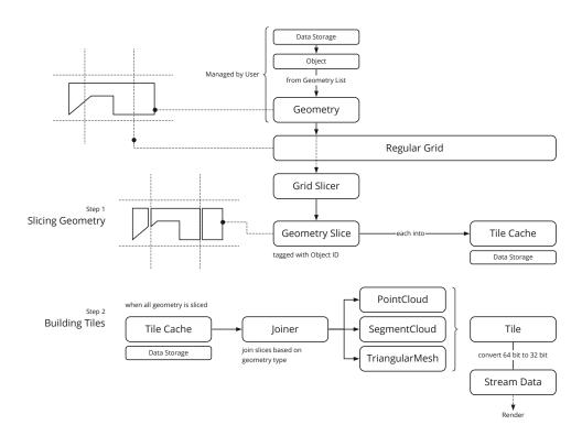
Figure 5.9: Grid Construction
