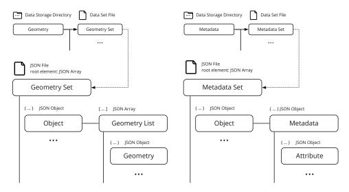
Figure 5.7: Example of Data Storage Contents
