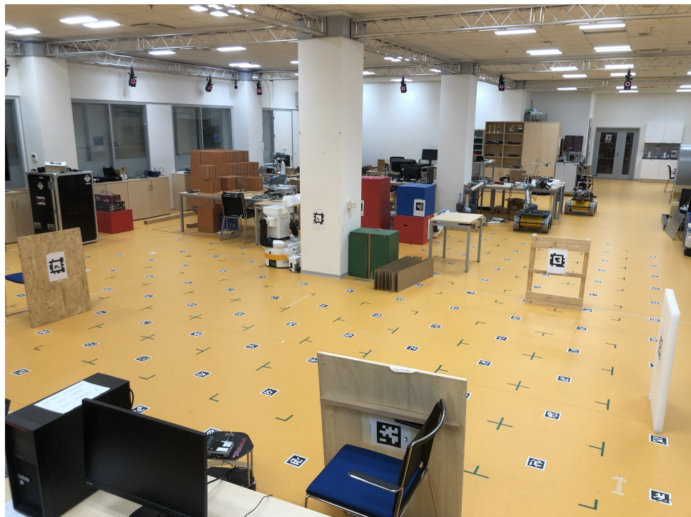
Figure 3.28: The large testing area with the Apriltags placed (approximately 30m^2 ).
