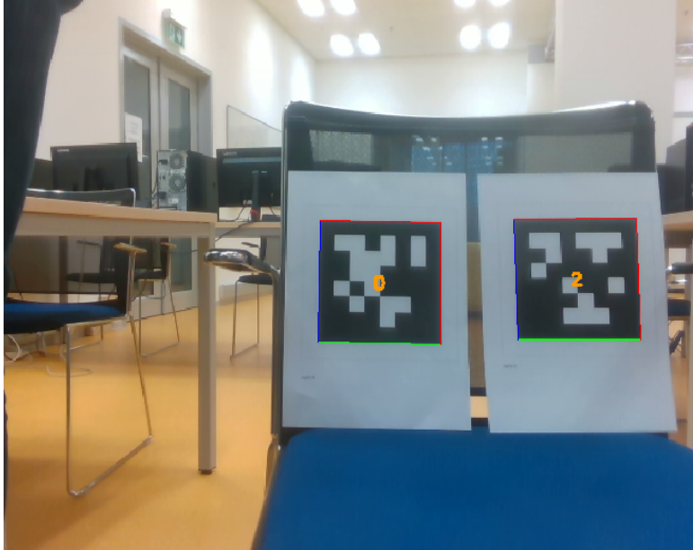
Figure 3.9: AprilTag detection via Intel RealSense D435 camera.
