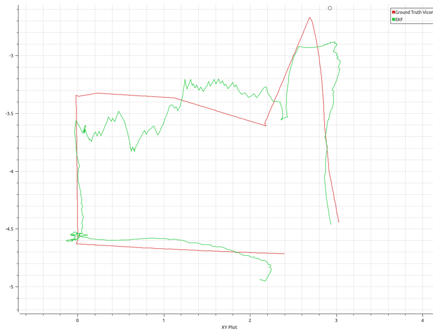
Figure 3.30: The two-dimensional trajectory (x and y axis) results are obtained from the larger environment test.
