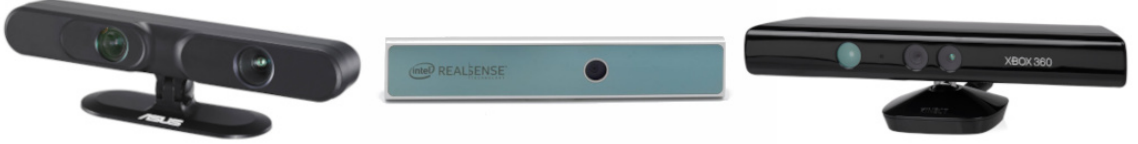
Figure 3.2: Examples of RGB-D cameras, based on the structured light technology. Left: ASUS Xtion Pro. Middle: Intel RealSense SR305. Right: Microsoft Kinect for Xbox 360.
