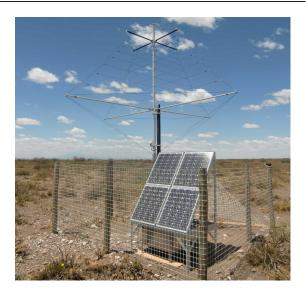
FIGURE 2. Photograph of an AERA radio-detector station.
