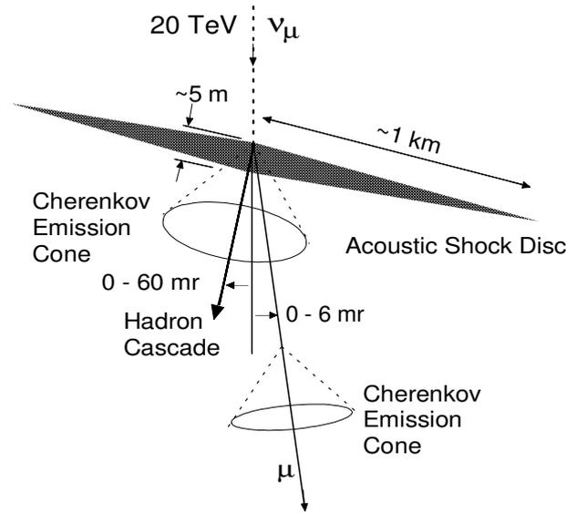
FIGURE 2. Characteristic effects caused by a high energy neutrino initiated interaction in a dense target medium. Analogous effects occur in  $\nu_e$  and  $\nu_\tau$  triggered reactions. Note that in principle the Cherenkov process generates optical as well as radio emission.
