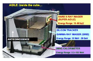
FIGURE 1. The AGILE payload.
