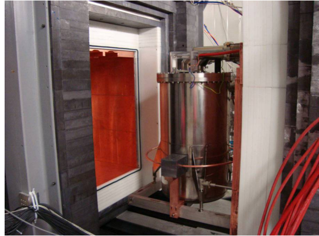
FIGURE 2. XENON100 with opened shield door. The circular copper pipe around the detector is used for inserting calibration sources from outside the shield. The Pb brick visible at the front is necessary to block gamma rays from the AmBe source during neutron calibration.
