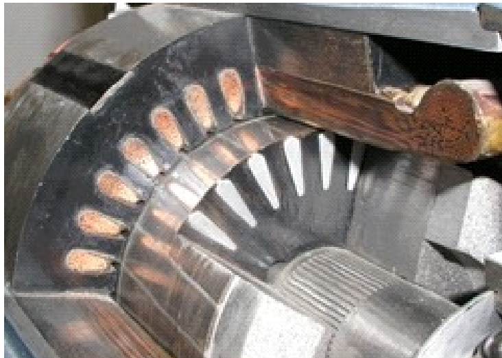
Fig. 6: Cutaway of small squirrel cage induction motor.
