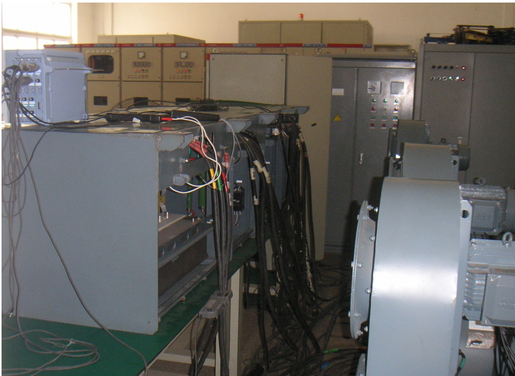
Fig. 60: Converter of the 180 kW machines test bench.
