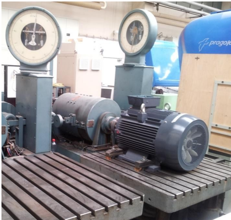
Fig. 53: 1AOE132MK-4 15 kW tested induction machine on a test bench stand.
