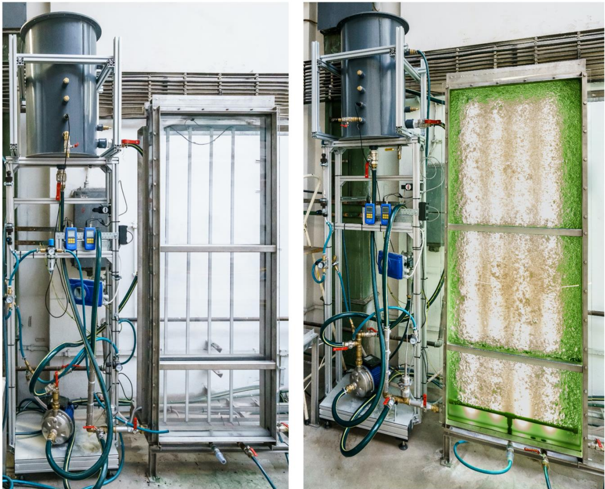
Fig. 7.1.1. Flat panel system installed in Department of Process Engineering laboratory.
