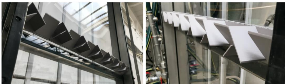
Fig. 8.1.3. Static mixer in FP PBR chamber.
