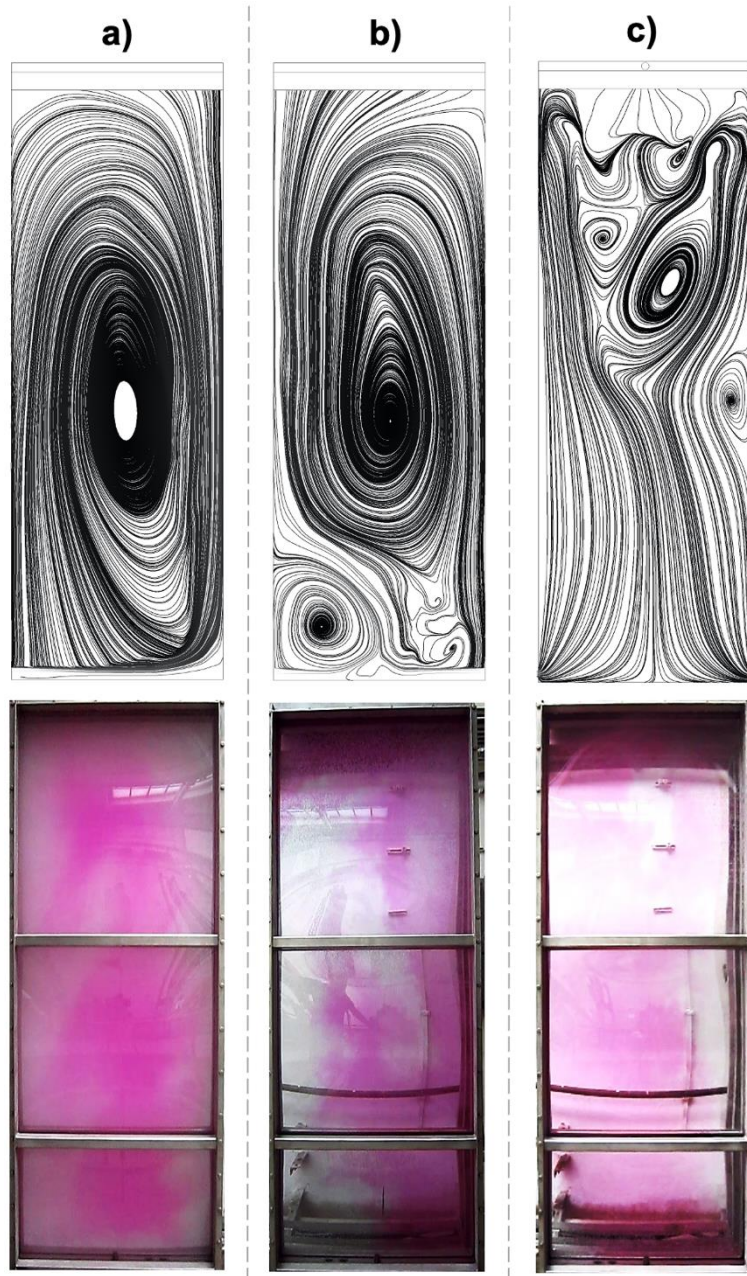
Fig. 7.2.2.3. Preliminary validation of CFD model. Comparison of tracer experimental measurement method (on the bottom) and numerical simulation of streamlines (on the top) – flow rate: 63 \text{ L min}^{-1} . a) single bottom inlet and top outlet, b) double bottom inlet and top outlet, c) top inlet and double bottom outlet.
