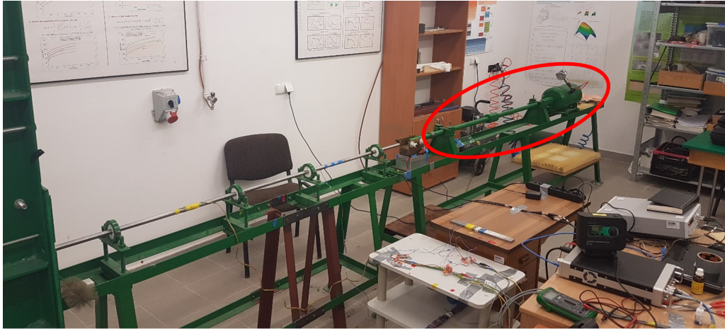
FIGURE 1. General view of the SHPB test stand DMEI (MUT) – on the right side of the test stand, there is a pneumatic launcher (the pressure chamber with the barrel are marked with a red ellipse).
