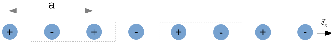
Figure 4.2: Two different choices of representative unit cells, indicated by the dashed lines, in a one-dimensional chain of alternating anions and cations. a is the lattice constant. Though both are valid, the unit cells present opposite polarizations.
