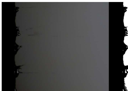
FIGURE 23. Original (left) and segmented (right) image using active contour method.
