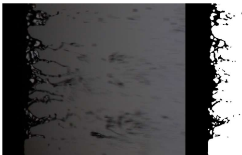
FIGURE 19. Original (left) and segmented (right) image using GMM-based method.
