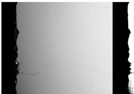
FIGURE 27. Original (left) and segmented (right) image using Otsu's method.
