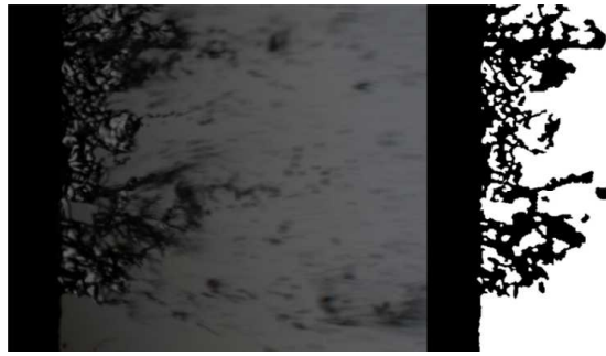
FIGURE 12. Original (left) and segmented (right) image using GMM-based method.
