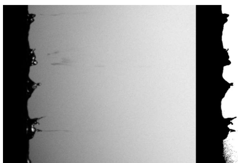
FIGURE 24. Original (left) and segmented (right) image using Otsu's method.
