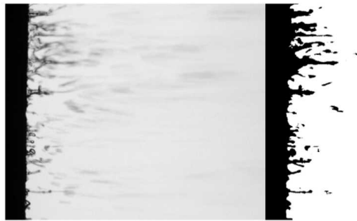
FIGURE 16. Original (left) and segmented (right) image using Otsu's method.
