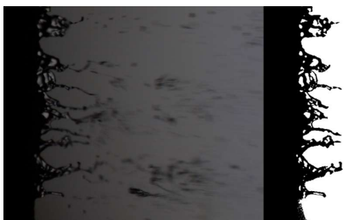
FIGURE 20. Original (left) and segmented (right) image using active contour method.
