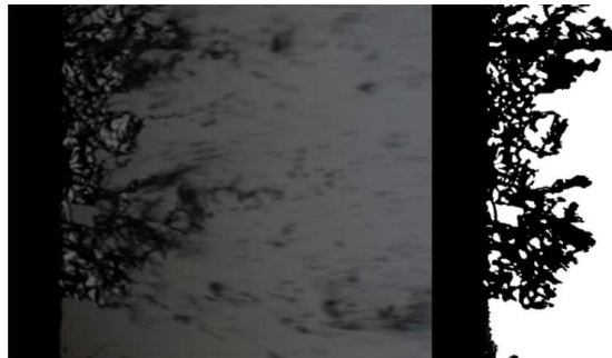
FIGURE 13. Original (left) and segmented (right) image using active contour method.
