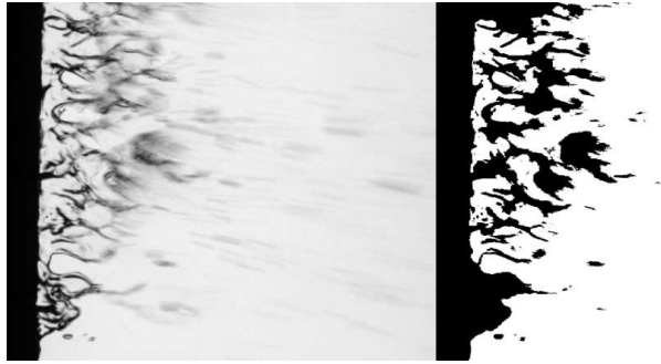
FIGURE 38. Original (left) and segmented (right) image using Otsu's method.
