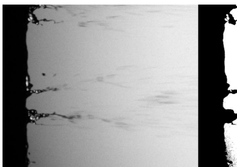
FIGURE 30. Original (left) and segmented (right) image using Otsu's method.
