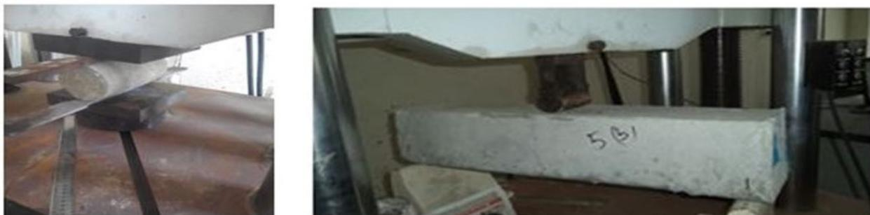
(E) . Splitting tensile strength test.
