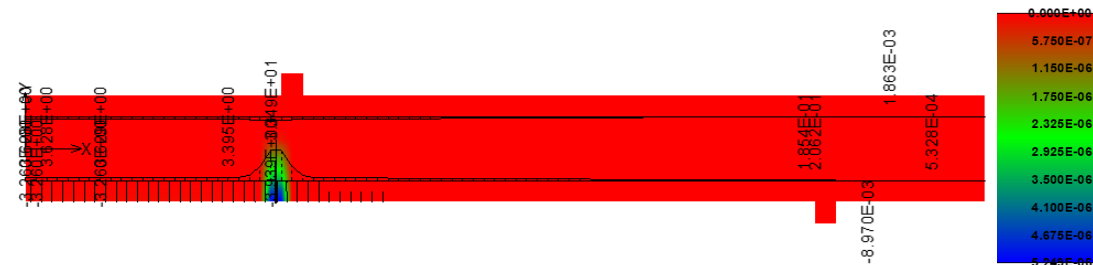
Fig. 119: Stress in the reinforcement after first crack opening and crack width (step 13).
