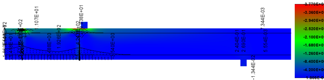
Fig. 94: Principal stress of concrete and reinforcement during the failure (step 210).
