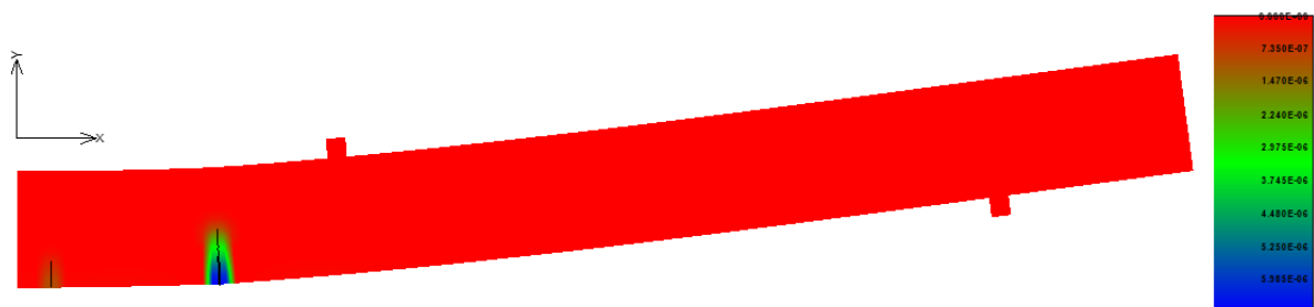
Fig. 56: Crack width after the first crack opening (step 15).
