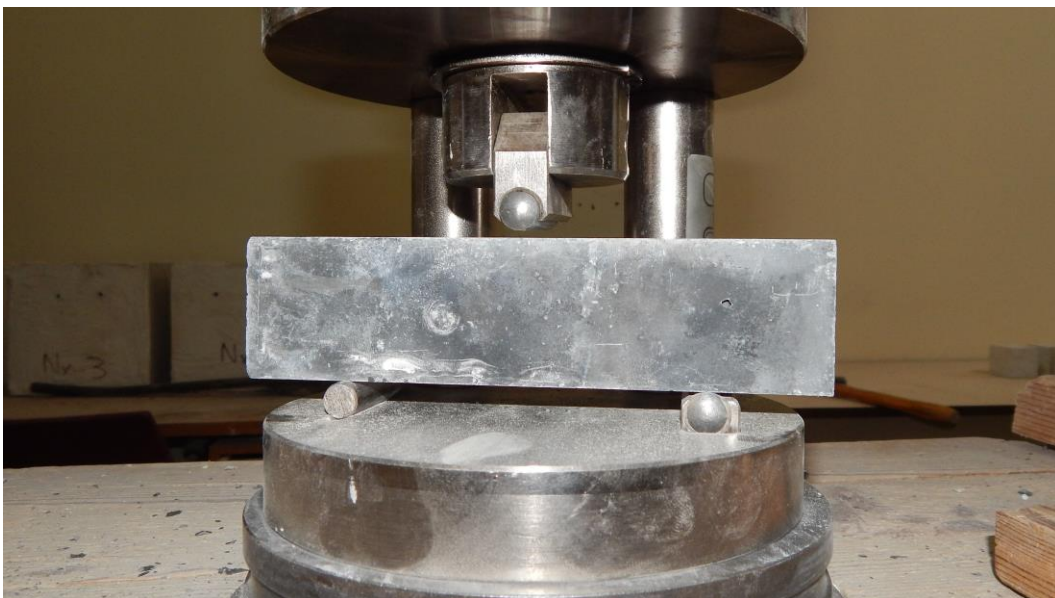
Fig. 8: Concrete prism with dimensions 40 x 40 x 160 mm just before testing procedure.
