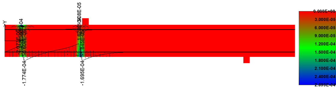
Fig. 96: Bond slip of the reinforcement and crack width (step 210).
