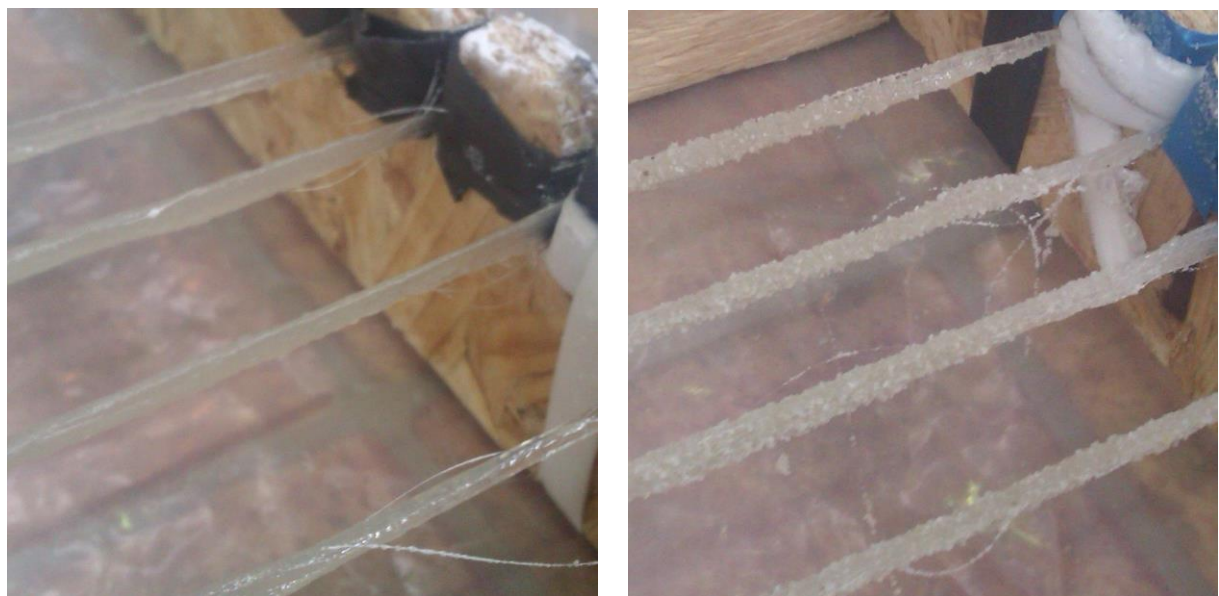
Fig. 4: Detailed view on impregnated single rovings without surface modification (left) and with surface modification using fine grain silica sand (right).
