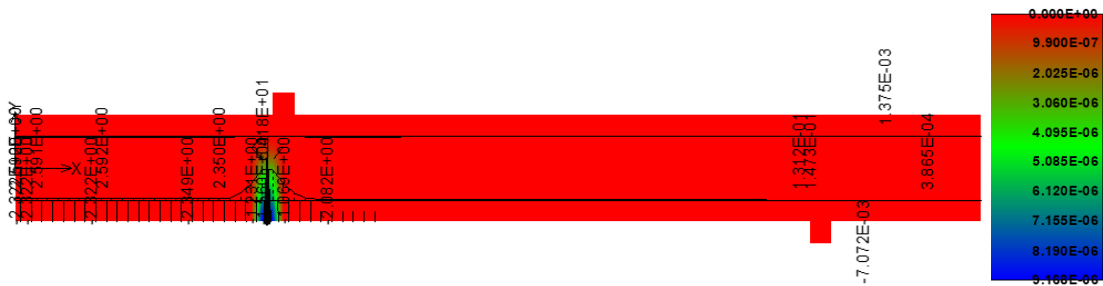
Fig. 137: Stress in the reinforcement after first crack opening and crack width (step 13).
