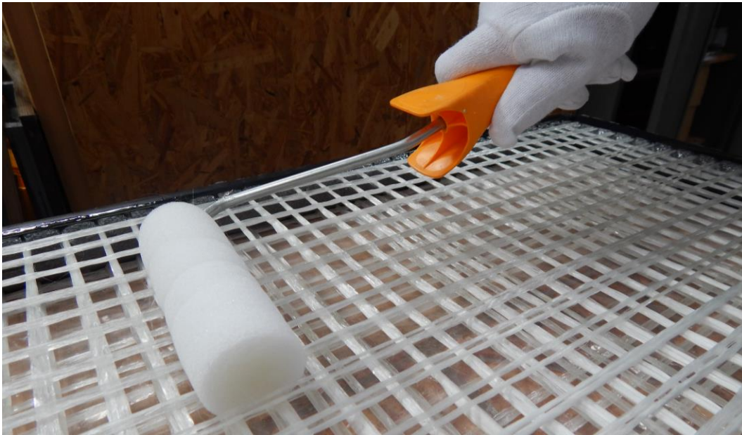
Fig. 2: View on the process of impregnation of own made textile reinforcement using epoxy resin and painting foam roller.
