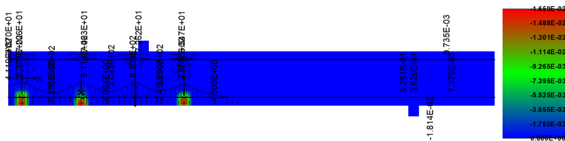
Fig. 105: Eq plastic strain of concrete and stress of reinforcement during the failure (step 120).
