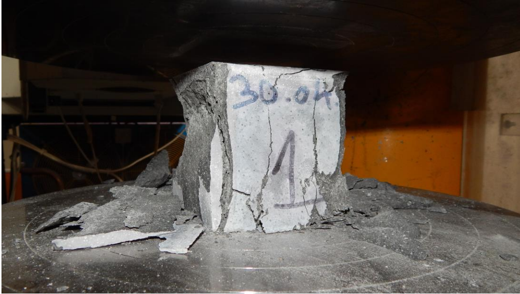
Fig. 7: Concrete cube with edge length 100 mm after the testing procedure.
