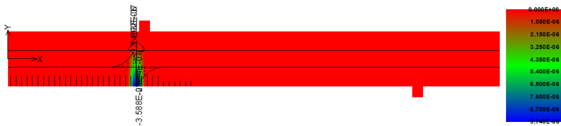
Fig. 111: Slip of the reinforcement after first crack opening and crack width (step 13).
