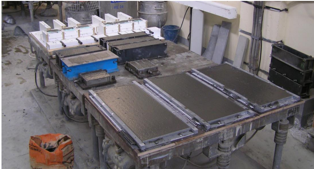
Fig. 1: More types of specimen just after the concreting and casting, pure HPC prism 40 x 40 x 40 mm, prisms 100 x 100 x 400 mm, cubes 100 x 100 x 100 mm, specimens for pull-out test 100 x 100 x 20 mm and façade TRC elements.
