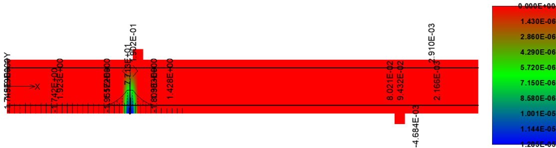
Fig. 101: Stress in the reinforcement after first crack opening and crack width (step 13).
