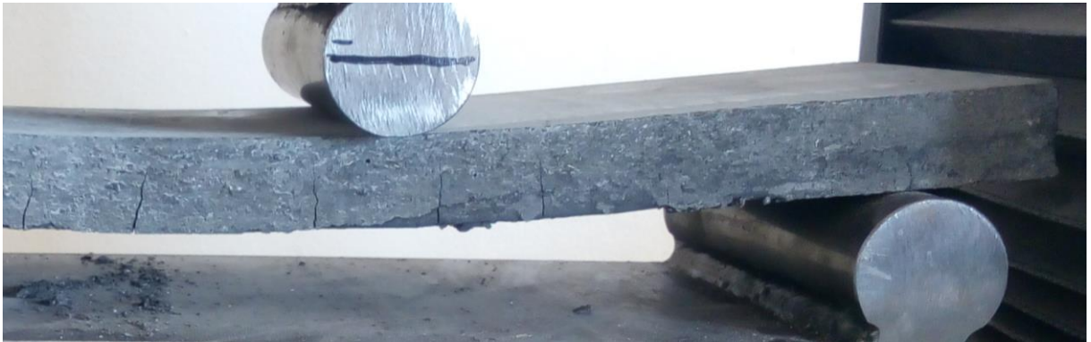
Fig. 121: Principal strain before failure of the structure (step 245) and below comparison of model with picture from the measurement, visible multiple cracking.
