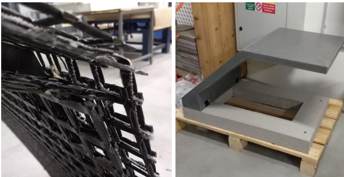
Fig. 150: Detailed view on the TT of upper part in the area of L shape (a), view on the complete concrete bench prepared for mechanical loading-bearing test (b) [13].
