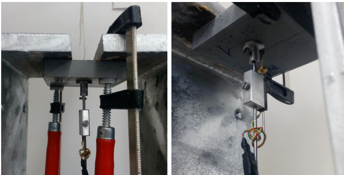
Fig. 23: Detailed view of bottom part of concrete specimen with installed potentiometer and supported constructions for the pull out values measurement
