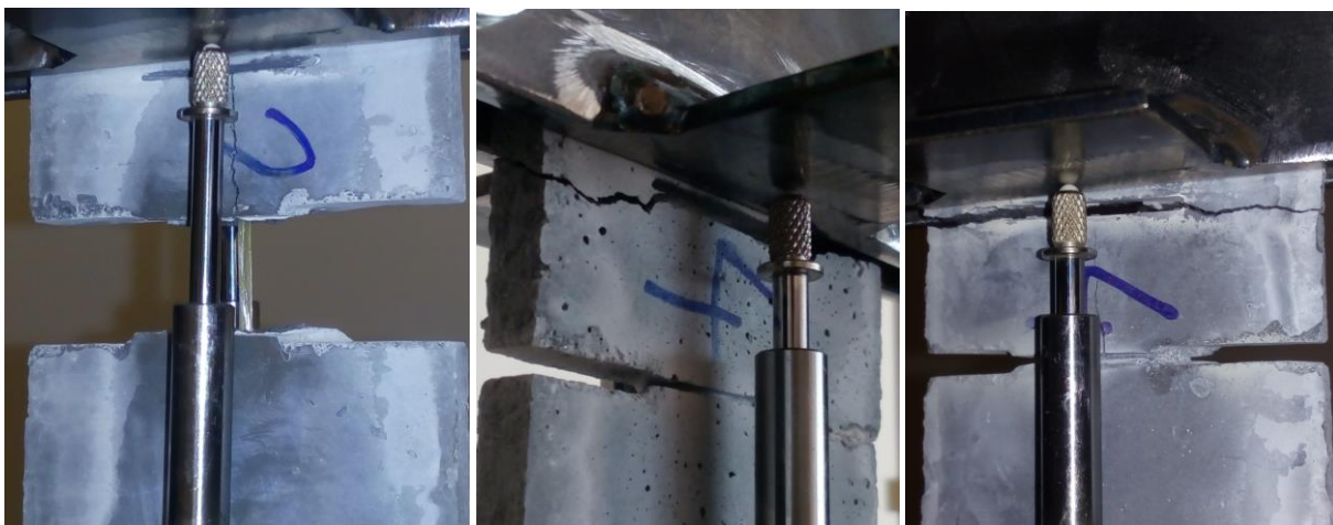
Fig. 20: View on the damaged specimens, smooth roving with typical vertical crack (left), smooth roving with typical horizontal crack (middle), roving with surface treatment and typical both vertical and horizontal crack (right).
