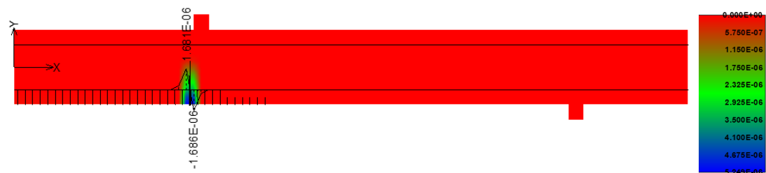
Fig. 120: Slip of the reinforcement after first crack opening and crack width (step 13).
