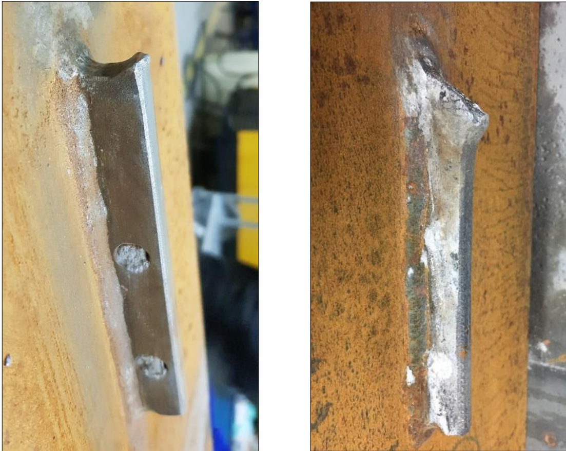
Obr. 124 Detaily deformace lišty
