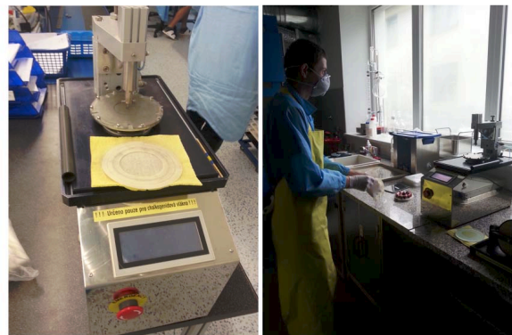
Fig. 5. Working station for soft-glass fiber modules polishing (right), a specialist in protective suit (right).
