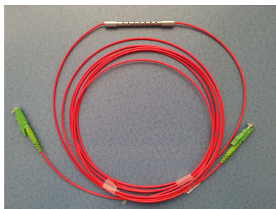
Fig. 3. TOF sensor sample encapsulation in protective metallic tubing, which allows liquid through-flow, equipped with E2000 connectors for easy inclusion in any optical system.
