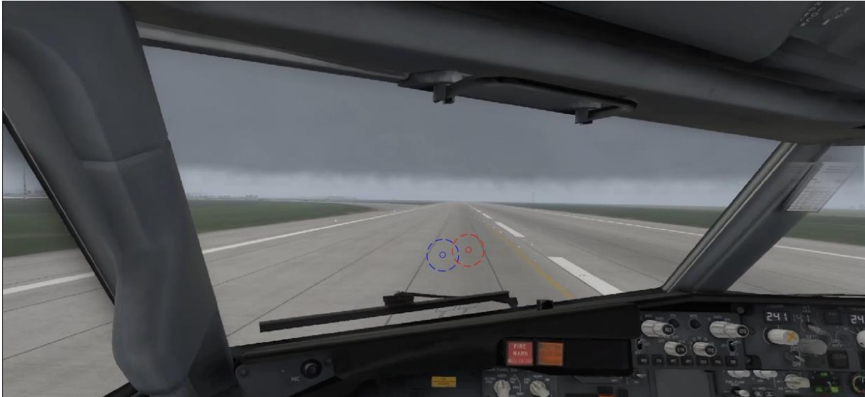
Figure 10. Primary Field of View in Measurement Video with Eye tracking Overlay (Blue – Left Eye, Red – Right Eye)
