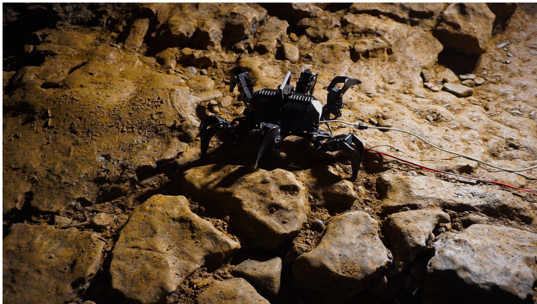
Figure 3: Hexapod walking robot SCARAB (Slow-Crawling Autonomous Reconnaissance All-terrain Bot) in the underground environment.
