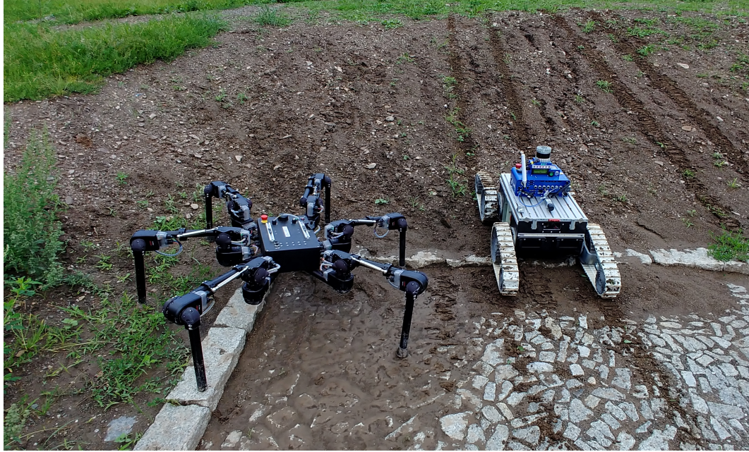
Figure 2: Differences between the impact of a legged robot (Lily the hexapod robot by HEBI Robotics) and tracked robot (MARV by Jettivision) on the sloped muddy terrain.
