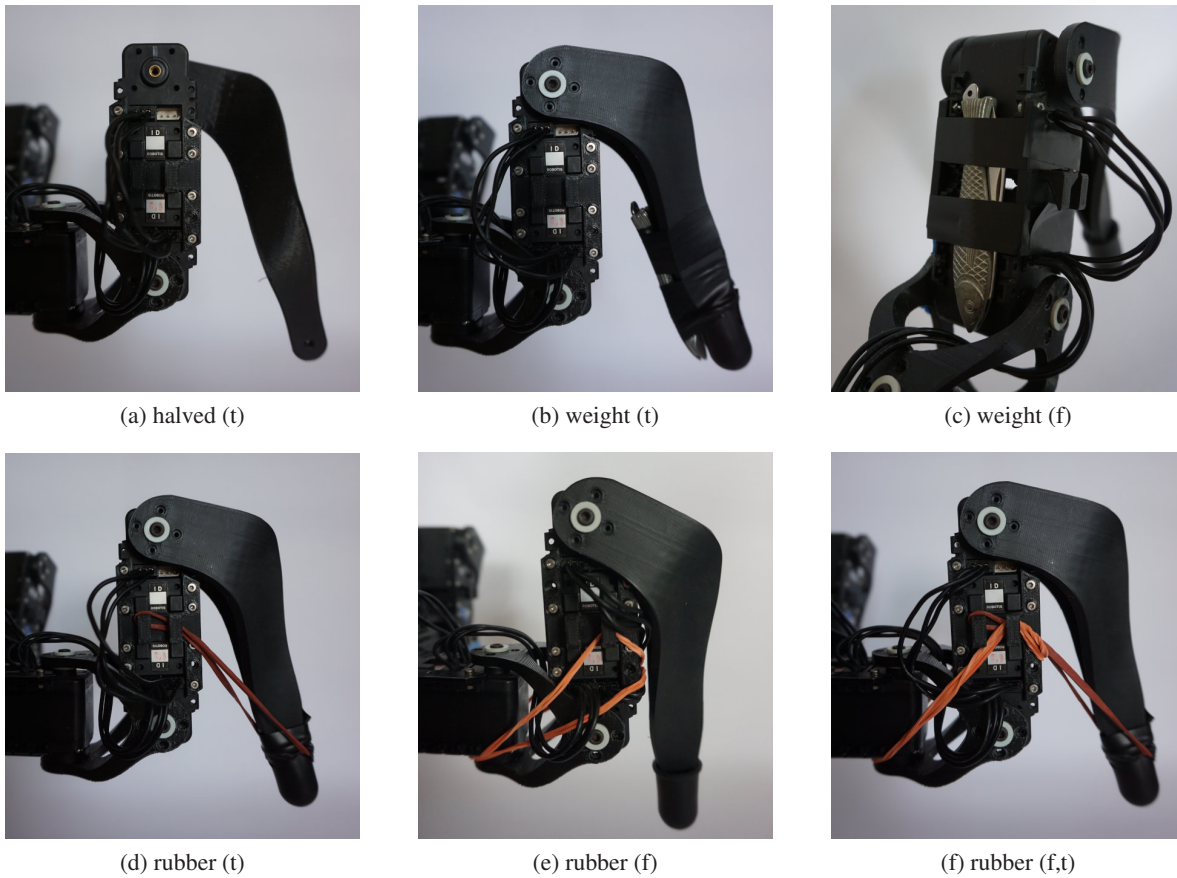
Figure 12: Leg modifications to introduce additional non-stationarities and alter leg parameters.
