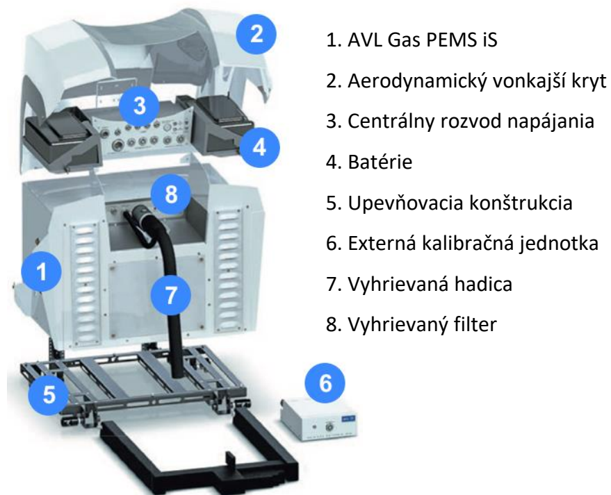
Obr. 6.3: Popis AVL M.O.V.E Gas PEMS iS [26]
