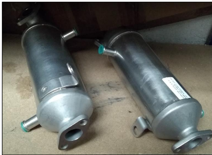
Figure 40 EGR Cooler 25.4mm Diameter Inlet/Outlet
