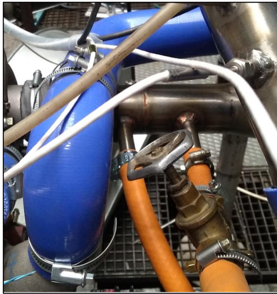
Figure 22 Common Mixer Fuel Injection System
