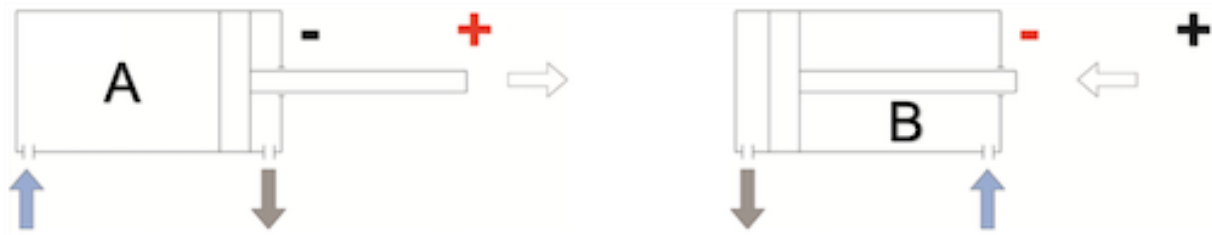
Figure 20 Pneumatic Piston Motion
