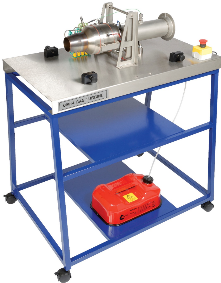
Figure 3.1 CM 14 axial gas turbine setting, source: armfield.co.uk
