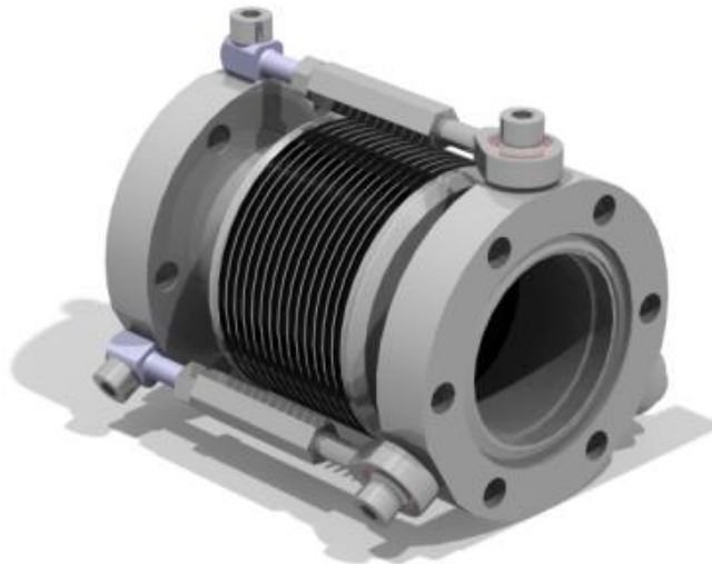
Fig. 21: Edge welded bellow with pivot mounts as an aligner [48]
