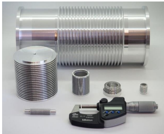
Fig. 22: Metallic mandrels for electroforming (NiCoForm) [51]
