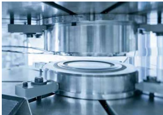
Fig. 16: Stamping tools mounted on the machine (Comvat AG) [42]
