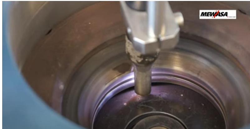
Fig. 18: Edge-welding of inner diameter of two diaphragms (Mewasa AG) [43]
