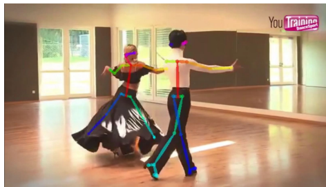
(e) : Body parts detection failed and proposed parts of the skirt as candidates for the knees and feet.
