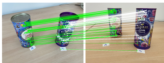
Figure 5.2 An image pair with two dominant objects. Green and white correspondences connected with lines are inliers of two fundamental matrices. The object "A" (cylinder in the left) was deliberately moved to create two possible structures for epipolar geometry estimation, while the correct \mathbf{F} is the one having white matches.
