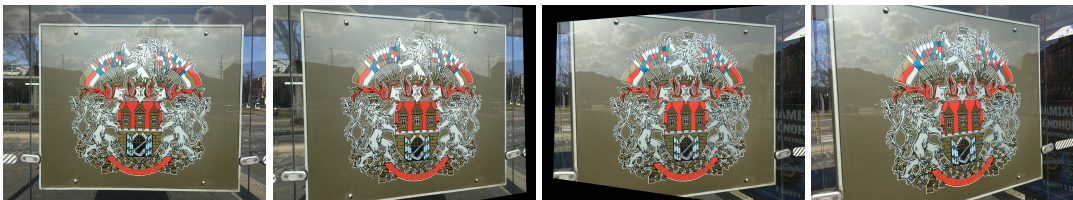
Figure 7.1 The left most image is a reference, the right most is a destination. Two images in the middle (supposed to be the same) represent "half" homography transformation from the reference to destination and vice-versa . The second image was generated by projecting points of the destination image by the inverse of square root of homography, and the third image was generated by projecting points of the reference image by the square root of homography.
