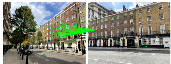
Figure 2.4 Homography estimation on an image pair sharing no common scene matched by SIFT detector. Green circles (95) are points consistent with the final model, the only red one – independent inlier. The model is predicted to be random.
