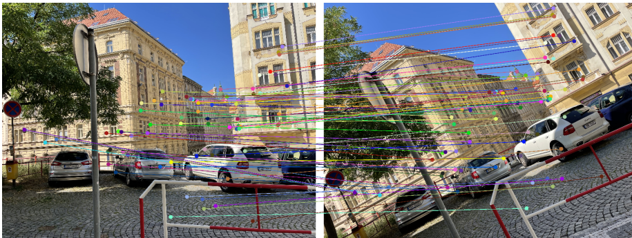
Figure 3.5 An image pair of a scene without camera translation demonstrates matches (colorful circles) related by homography conjugated to rotation. This case was detected by the proposed in this section test.
