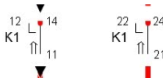
Figure 30. Two changeover switches
