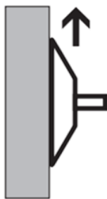
Figure 24. Vertical suction cup position with vertical movement (8)
