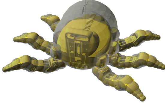
Figure 8: Sphere-based robot collision model approximation.
