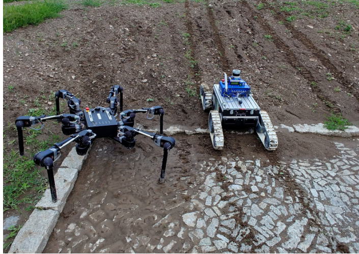
Figure 2: Example of the terrain traversed by hexapod walking robot and tracked robot. There are visible footprints of the tracked robot, while the legged robot does not make any significant marks when crawling over the sloped terrain.
