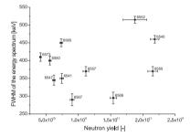
Figure 8: Dependence of the FWHM of the reconstructed energy spectrum on the total neutron yield.
