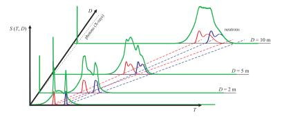
Figure 2: Propagation of a long duration neutron burst through the free space (green signals). Two elementary short pulses (red and blue) are indicated to show the superposition of spectra of neutrons which were emitted at various times. The signals were normalized to the same height.
