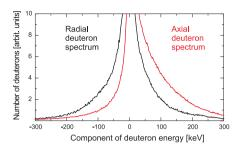
Figure 13: Kinetic energy components of reacting deuterons, shot No. 090922. The plus and minus signs of kinetic energy component reflect the direction of a deuteron velocity.
