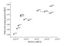
Figure 7: Dependence of the mean energy of the reconstructed energy spectrum on the total neutron yield.
