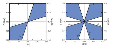
Figure 3: Reconstruction plane, i.e. a time-resolved energy spectrum, with the angles of the direction of sight for the minimum and maximum distances of the detectors.
