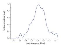
Figure 5: Neutron energy spectrum received by an integration of time-resolved energy spectrum from Fig. 4 (shot No. 6540).
