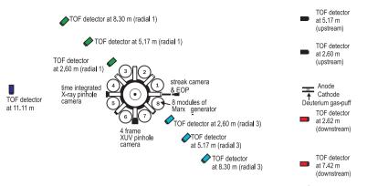
Figure 9: S-300 device – a schematic diagram of the diagnostic setup (left: end-on view, right: side-on view) with 11 time-resolved hard X-ray and neutron detectors (September 2009).
