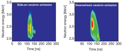
Figure 11: Neutron energy spectra in the side-on (radial) and end-on (axial) directions, shot No. 090922.
