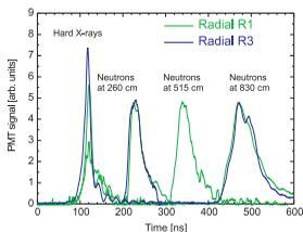
Figure 10: Side-on TOF signals (shifted by the TOF of X-rays, shot No. 090922).
