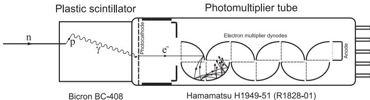
Figure 1: Two main parts of the scintillation detector – a scintillator and PMT.
