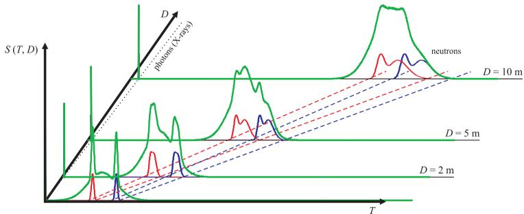
Figure 2: Propagation of a long duration neutron burst through the free space (green signals). Two elementary short pulses (red and blue) are indicated to show the superposition of spectra of neutrons which were emitted at various times. The signals were normalized to the same height.
