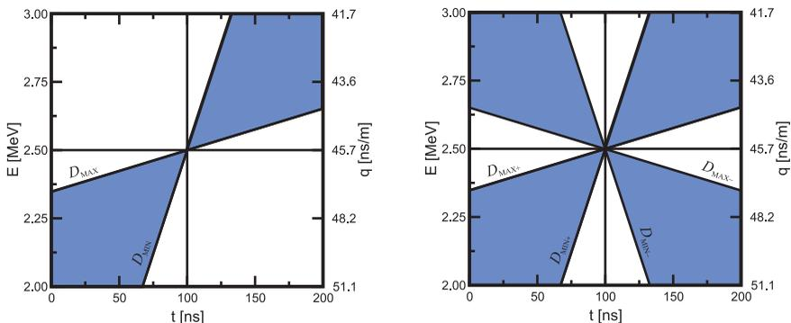
Figure 3: Reconstruction plane, i.e. a time-resolved energy spectrum, with the angles of the direction of sight for the minimum and maximum distances of the detectors.
