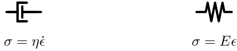
Figure 4.1: Two most commonly used elements for describing viscoelastic models, a dashpot on the left and a spring on the right.
