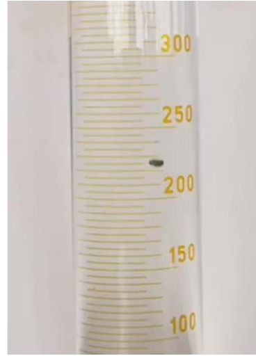
Figure 6. Illustrative image of a feed pellet settling in a water column
