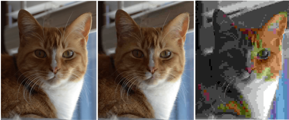
Figure 2.16: Example of JPEG compression. (Left) raw, uncompressed image, (middle) medium level compression, perceptually lossless, (right) highly compressed image. Adapted from [40]
