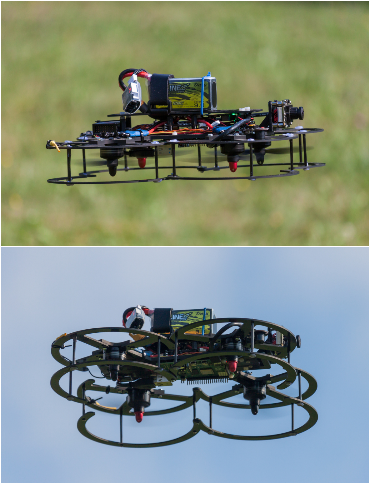
Figure 3.5: Detail photos of the real model during experimental flight. The model is equipped with all necessary sensors, including VIO camera.
