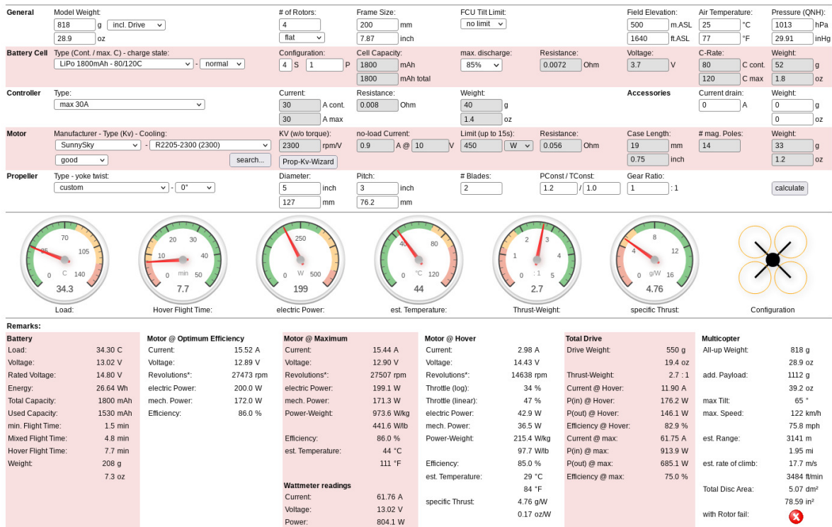
Figure 3.3: Result of eCalc design of the drive components and its flight characteristics.
