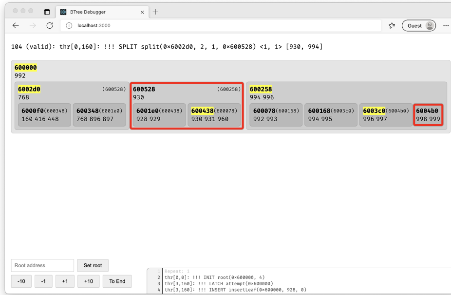
Figure 5.1: Web based visual debugger displaying the internal state of a tree. Red boxes denote split nodes not yet inserted to the parent node. A highlighted node address indicate that a thread has latched that node.
