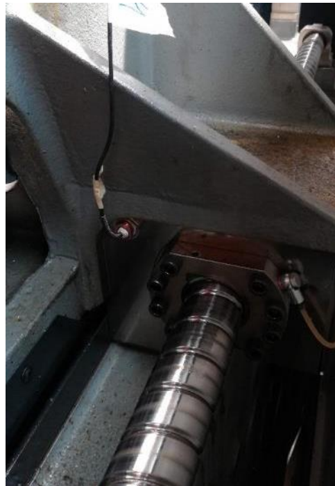
Fig. 14 External temperature sensor placed on the dynamic element (front side of the ball screw nut).
