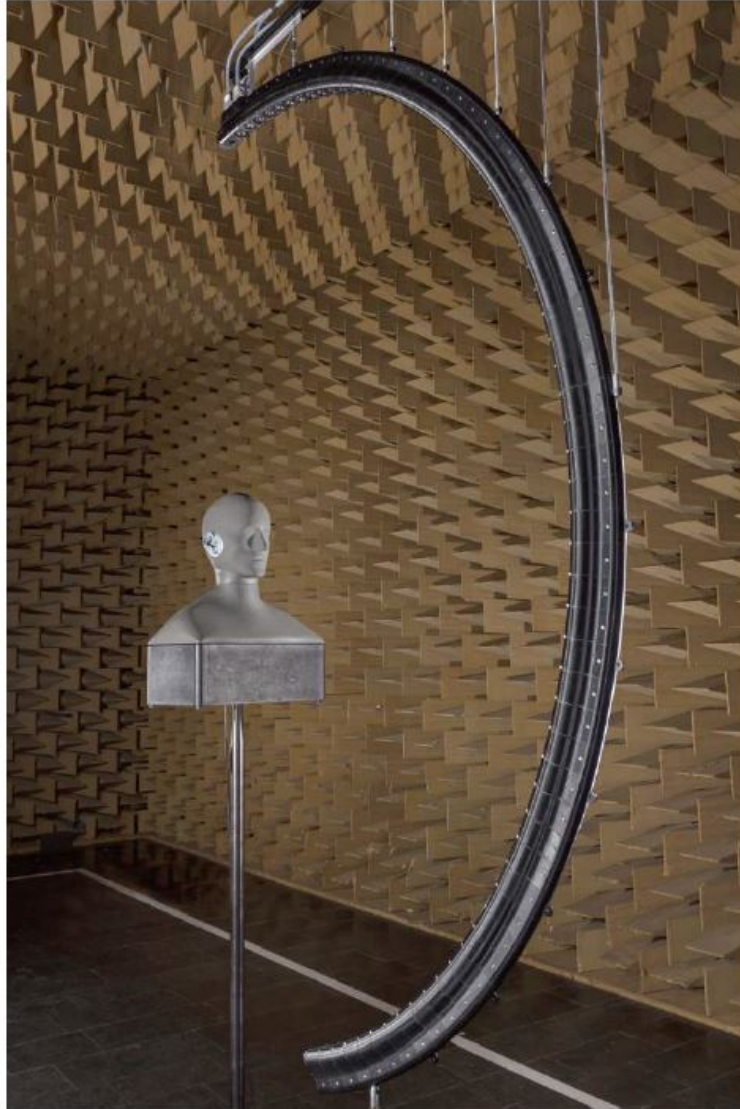
Figure 3.2. The HRTF measurement arc of the Institute for Hearing Technology and Acoustics. The IHTA artificial head is used for the measurement. (Taken from [6].)
