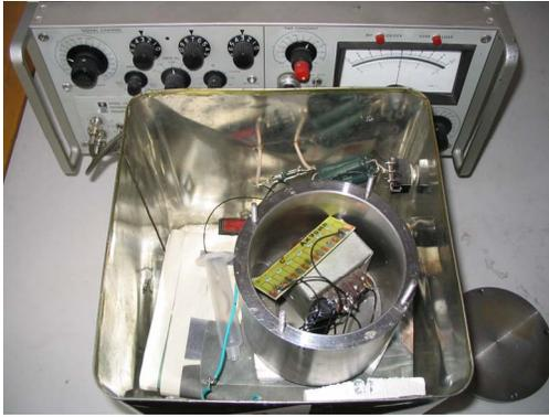
**Fig. 4** The measurement of noise. Behind the screening box is the lock-in amplifier PAR 124 A.
