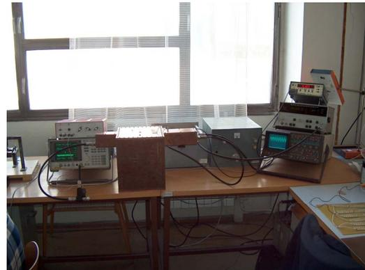
**Fig. 2** The working place for the measurement of nonlinearity of the I-V characteristics of the adhesive joints. The spectral analyzer HP 8560 is on the left, the power generator and filter in the middle, the oscilloscope and the second generator with the counter on the right.
