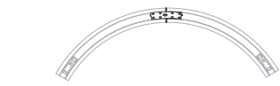
Code 2256010A_ JOINT 07a → 60° CURVE RIGHT - 60° CURVE RIGHT JOINT ← 60° CURVE LEFT - 60° CURVE LEFT JOINT
