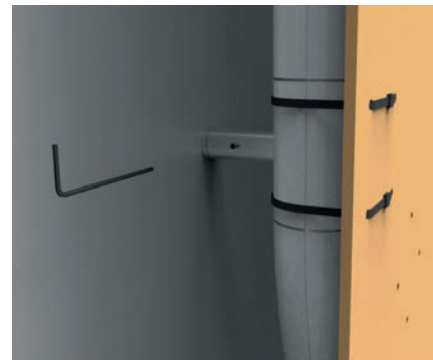
6. Detail of the wall pins fixing.
