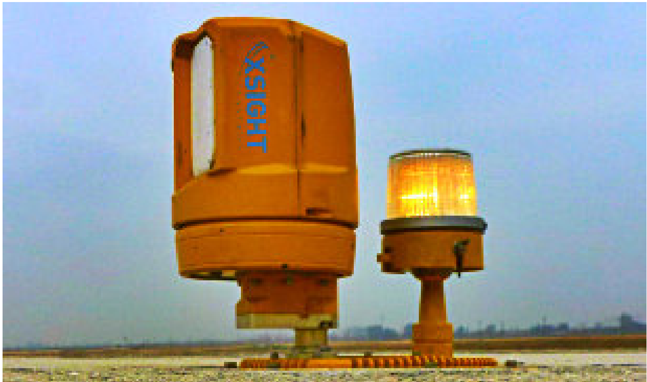
Figure 1.3: Example of an FOD detector combining radar and optical technologies [14]
