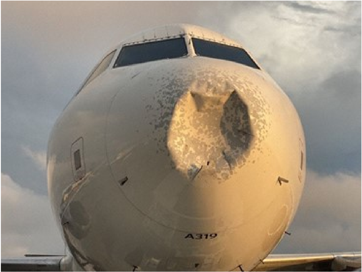
Figure 1.7: Damaged radome after flying through hail [26]
