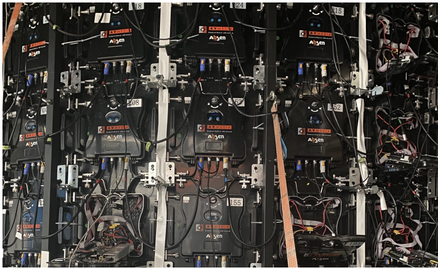
Figure 2.8: LED semi-curved screen back-side - LED segments
