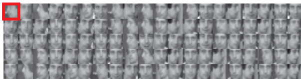
Figure 7. Online model obtained by the LOOP growing event contains examples that are very diverse but correctly represent the object. The LOOP exploits drift of adaptive trackers. The patch selected for tracking is denoted by the red square.
